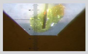
Embedded Si sample (perpendicular view with distance definition graticule)
