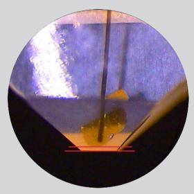
Perpendicular viewing for distance definition between sample and front face of the embedding material
